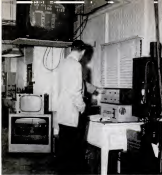
CLOSED-CIRCUIT TV SYSTEM lets men in tote room, down under the stands, keep a constant watch on the board. Cameras are controlled from the switchboard at the man's left hand.
